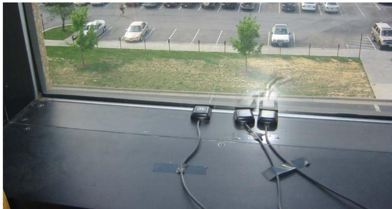
**Figure 1: Antenna placement inside window**
